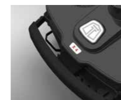
Sensor de parachoques y obstáculos blandos Bumper and soft obstacle sensor
